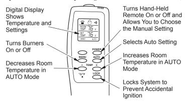
Figure 54 - Thermostat Hand-Held Remote Control Unit GHRCTB
